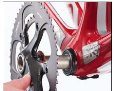
Figure 27. Sliding the axle through the bearings
